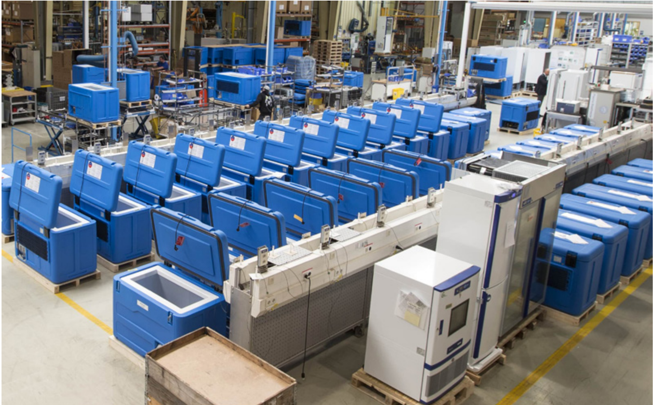
> View of the production plant with the assembly of the rotomolded components.
